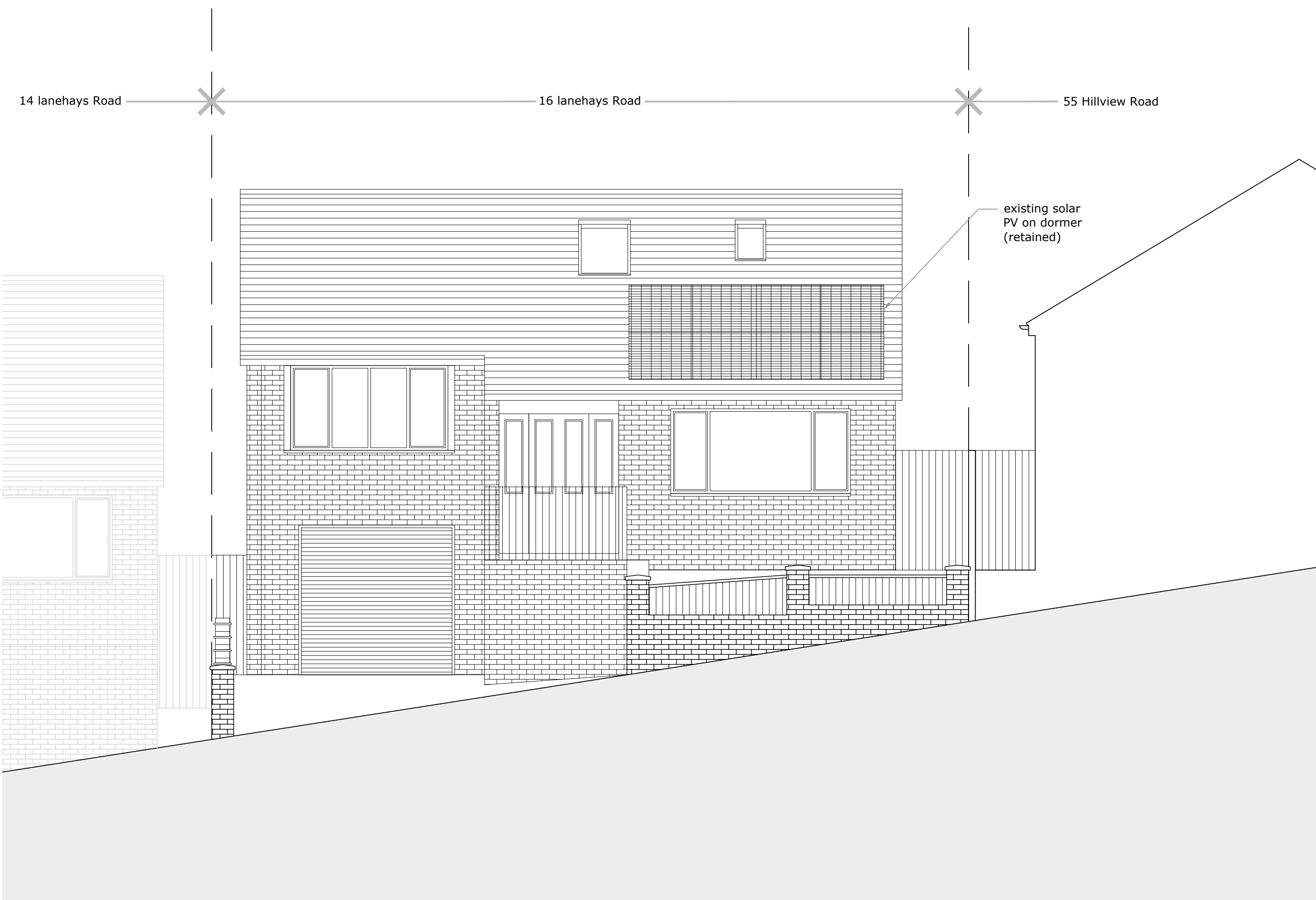
front elevation (west facing) as proposed 1:50
