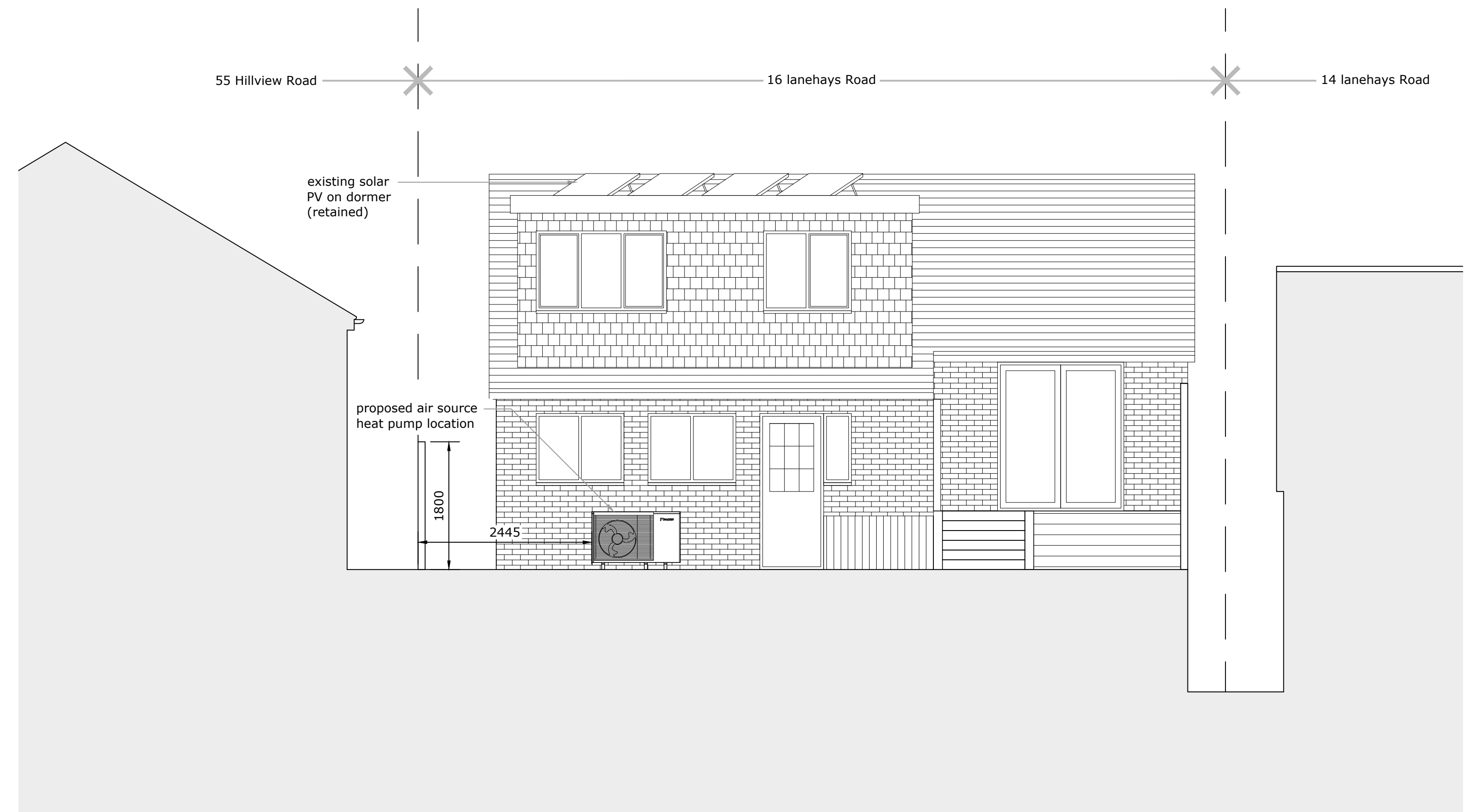
rear elevation (east facing) as proposed 1:50
