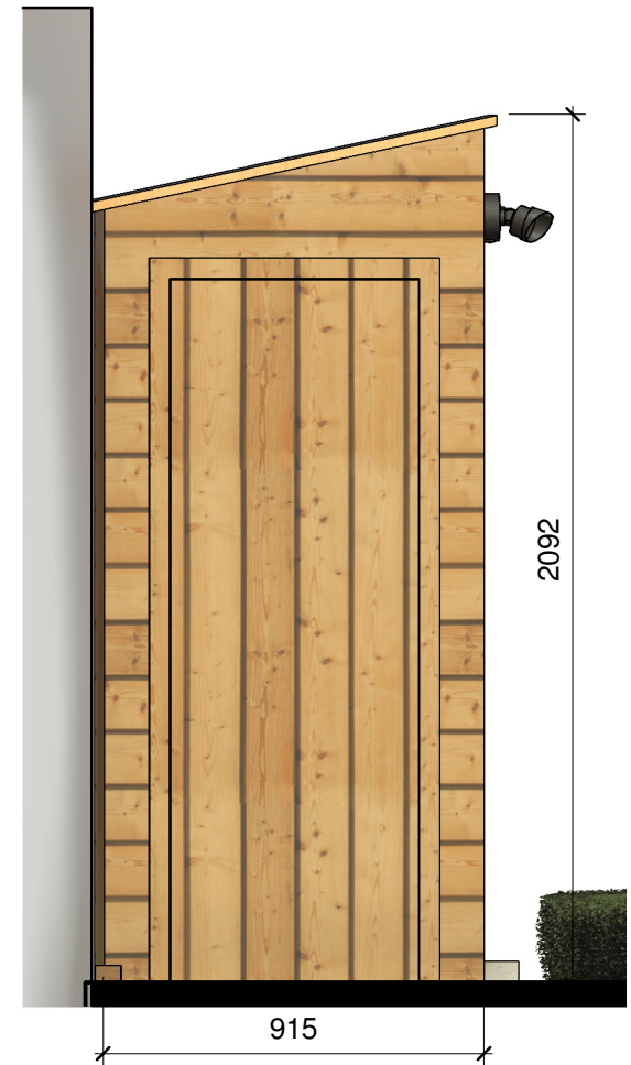
2 Timber Shed - Elevation 1 : 20
