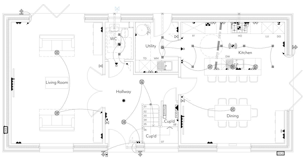
Switched fuse to be provided within meter box due to CCU distance from meter.
