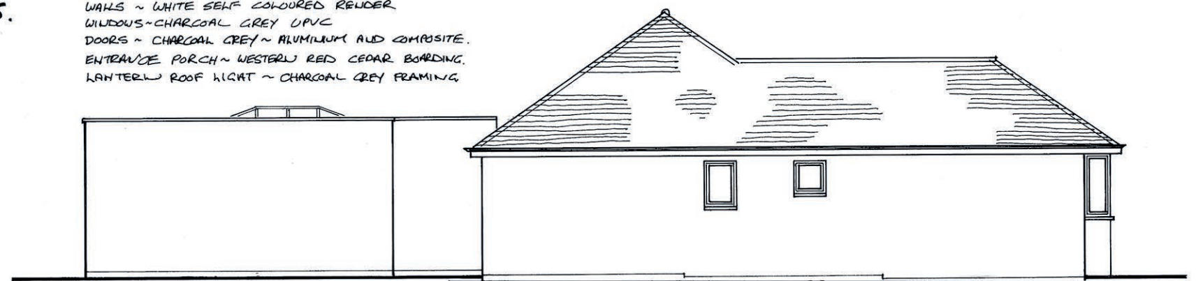
SIDE [NORTH] ELEVATION.
