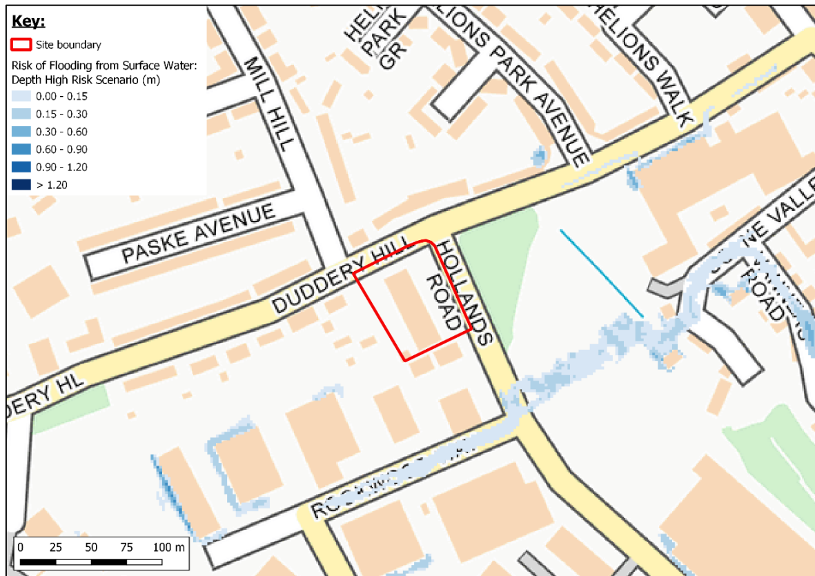
Figure 4.10 EA Risk of Flooding from Surface Water Map: Water Depth in High Risk Scenario (Contains Ordnance Survey data © Crown copyright and database right 2022 and public sector information licensed under the Open Government Licence v3.0)
