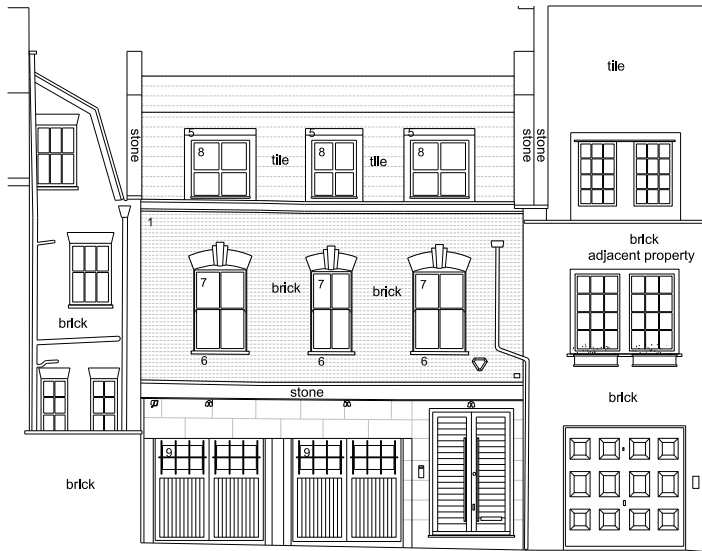
EXISTING FRONT - SOUTH ELEVATION 150 @ A1
