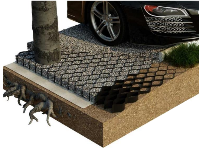
Fig. 5 Terram Geocell 20/20 load bearing surface for use in RPAs
