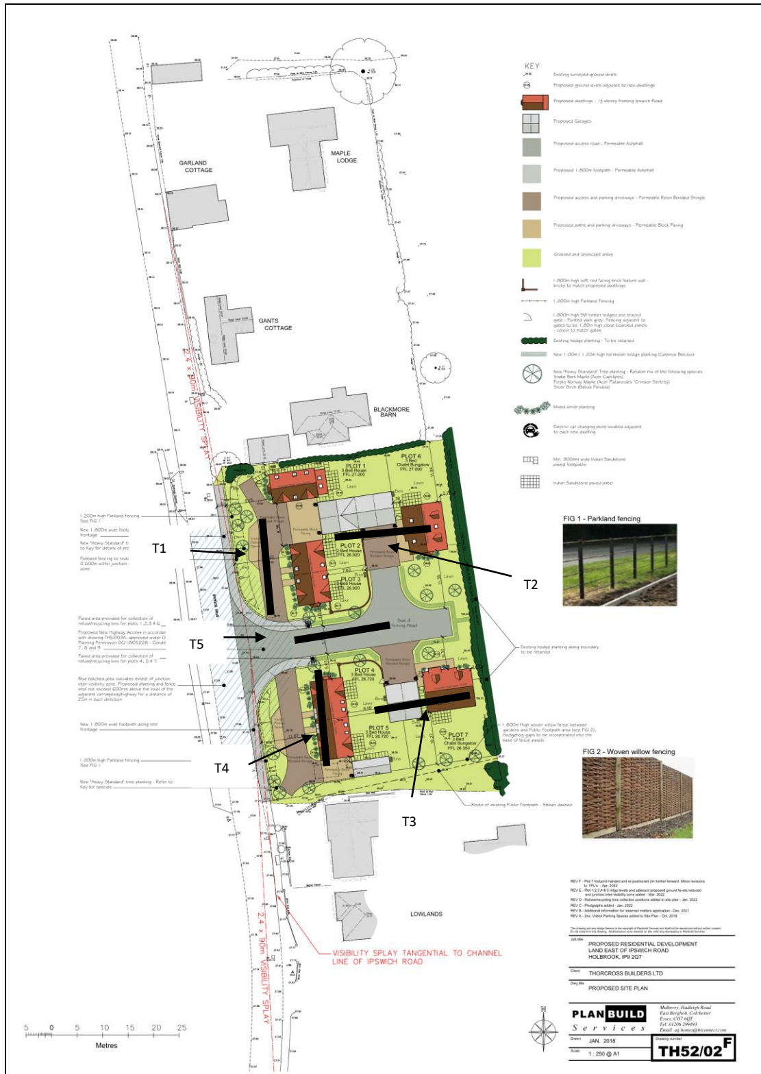
Location of trenches (5 x 20m)
