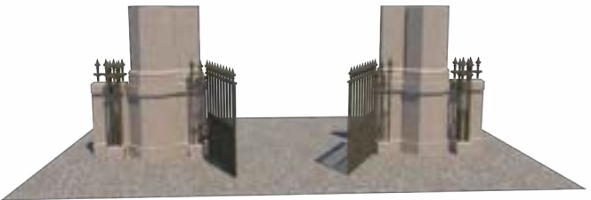
D Proposed Pedestrian Entrance x 2no. (India Gate) Note : Manual, free standing, single leaf gate
