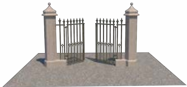
B Proposed Pedestrian Entrance x 2no. (New Road) Note : Manual, double leaf gate
