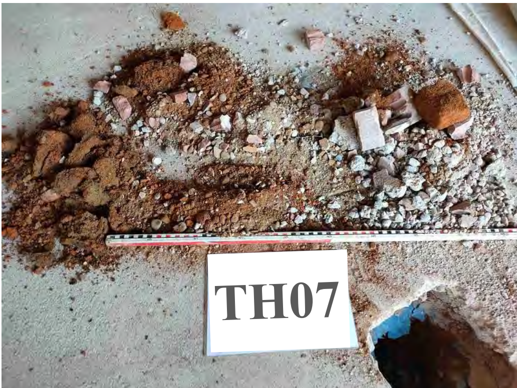
Plate 18: The arisings from trial hole TH07
