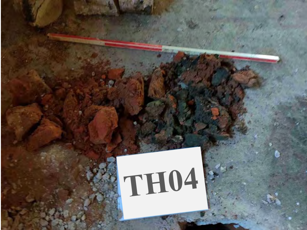
Plate 13: The arisings from trial hole TH04
