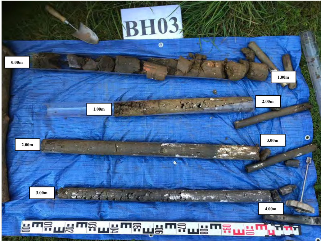
Plate 3: The arisings from borehole BH03, G.L. to 4.00m
