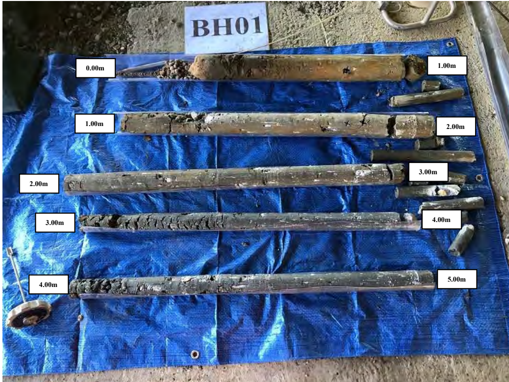
Plate 1: The arisings from borehole BH01, G.L. to 5.00m
