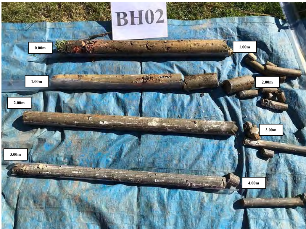
Plate 2: The arisings from borehole BH02, G.L. to 4.00m
