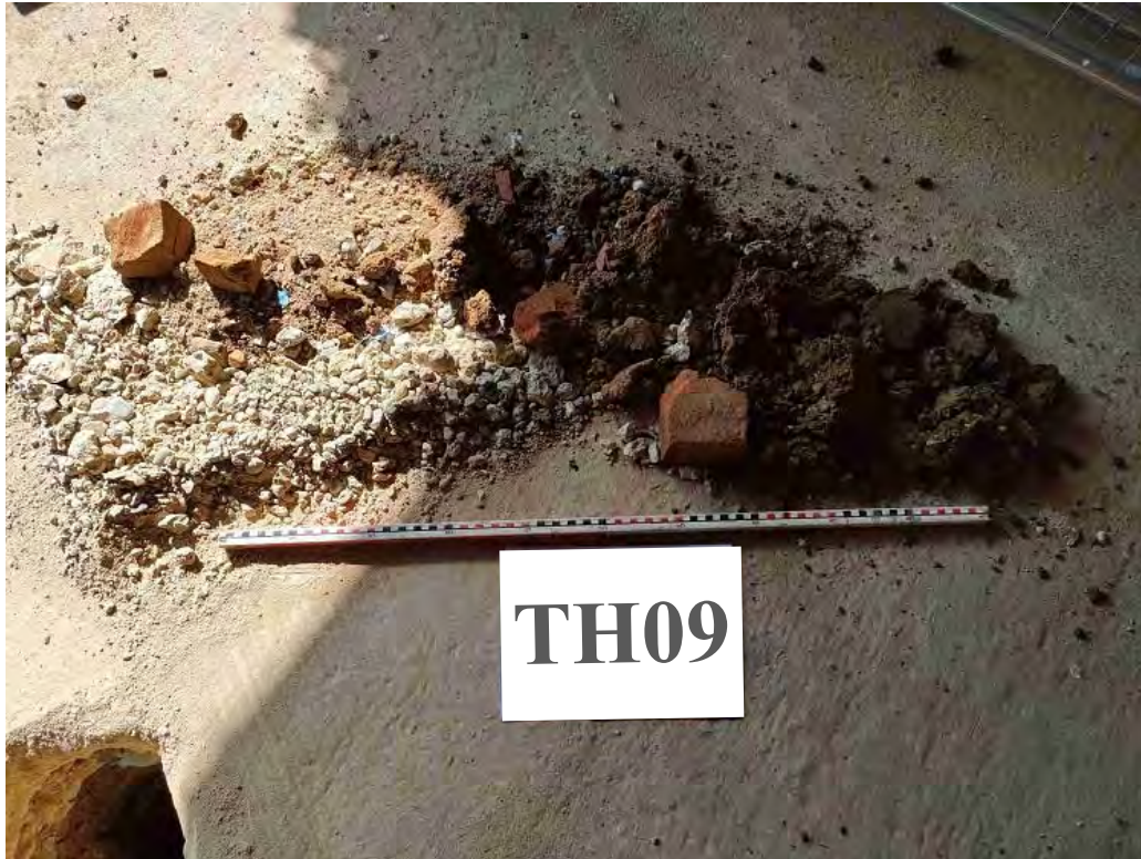
Plate 21: The arisings from trial hole TH09
