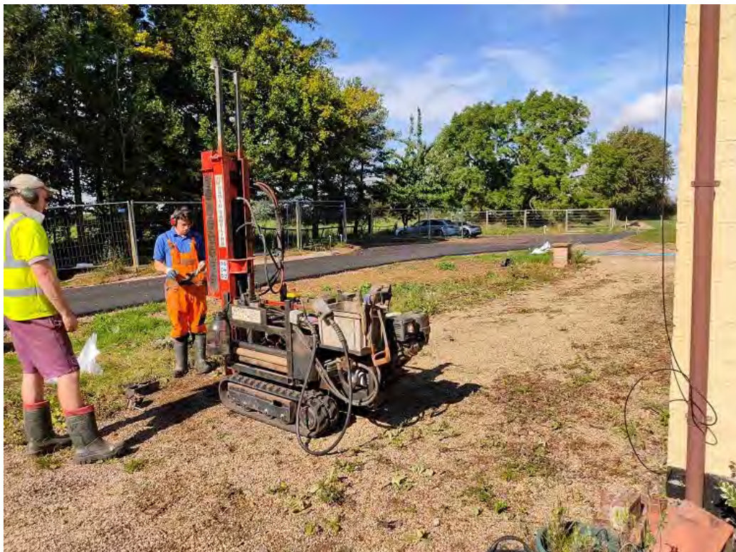
Plate 6: The Premier 110 window sampling rig on borehole BH04
