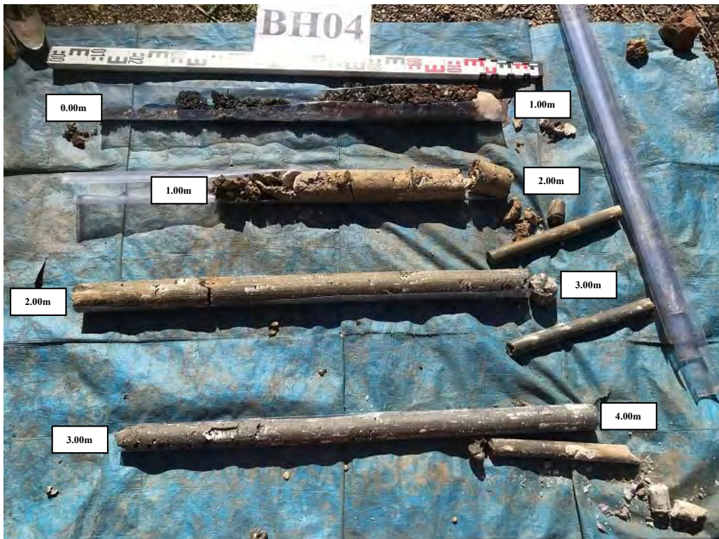
Plate 4: The arisings from borehole BH04, G.L. to 4.00m
