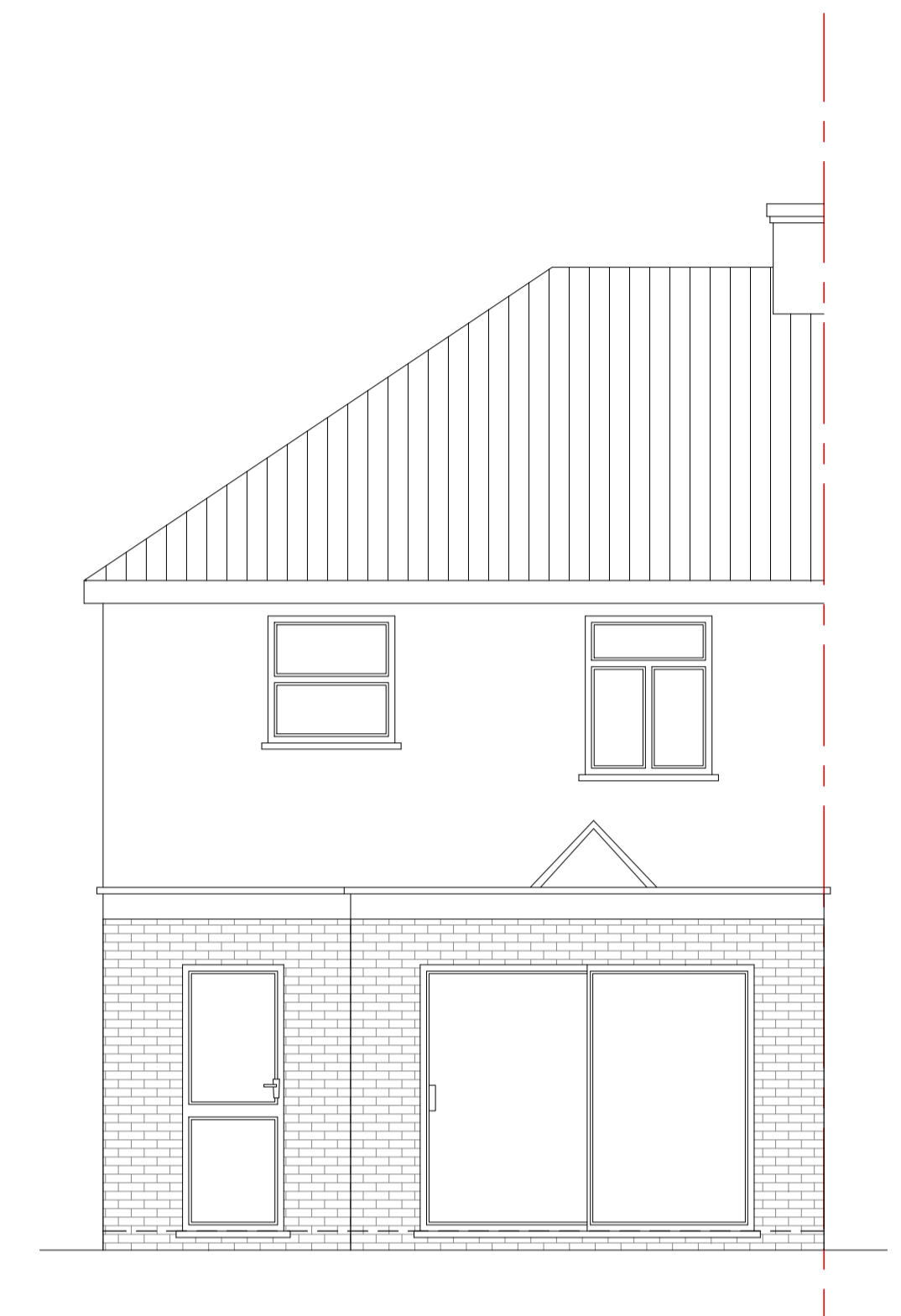
Proposed Rear Elevation 1:50
