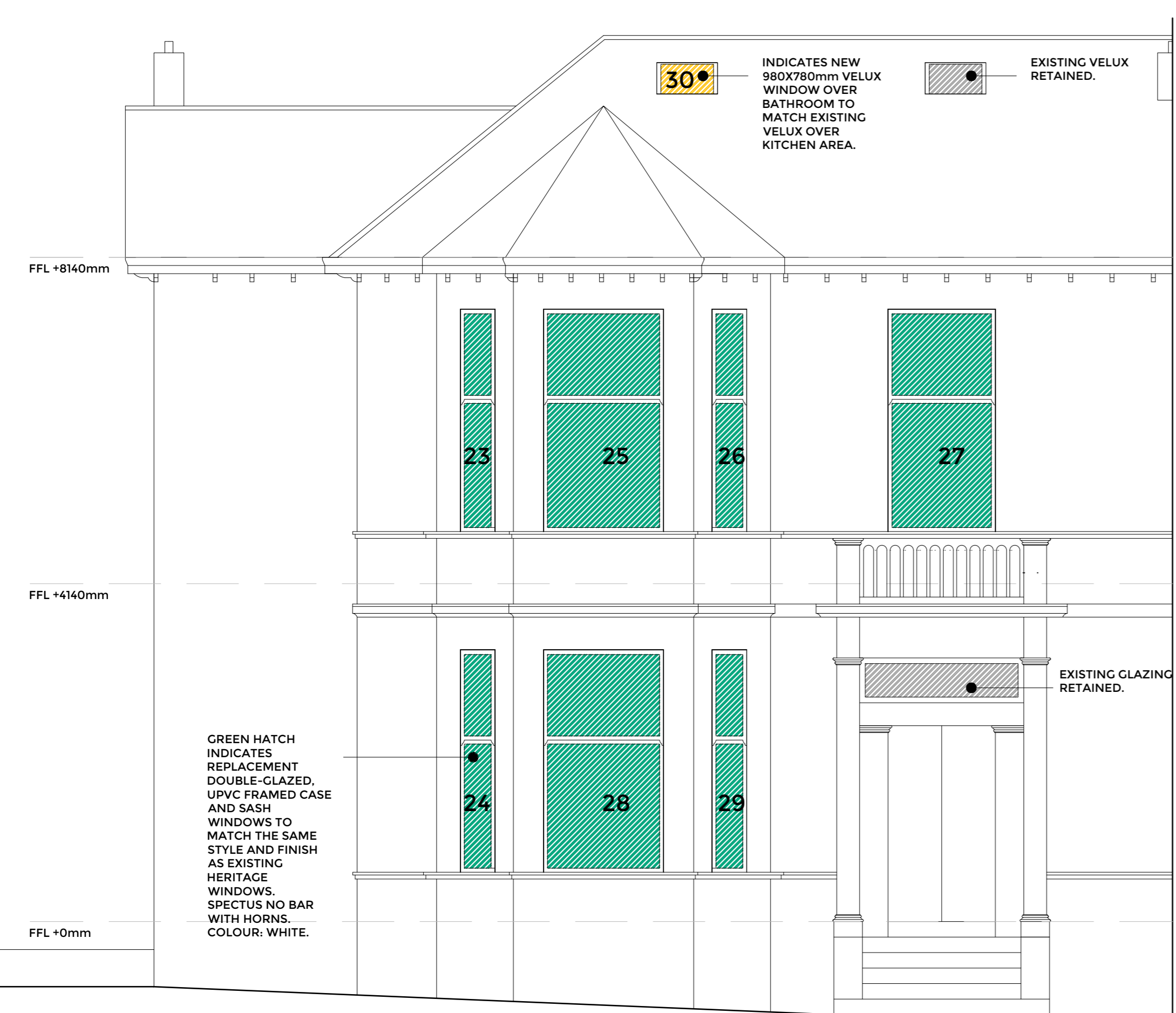
1m 0.5m WEST ELEVATION AS EXISTING
