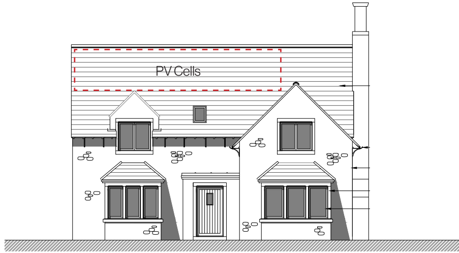
House 2 possible PV Cell location on southern facade
