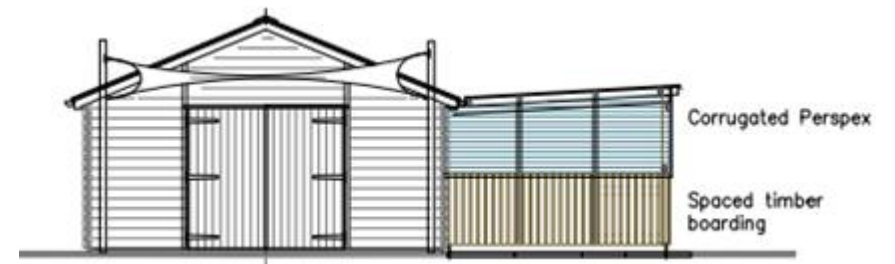
Figure 7 (above) Proposed Tea Shack principal (east) elevation (not to scale - indicative only)
