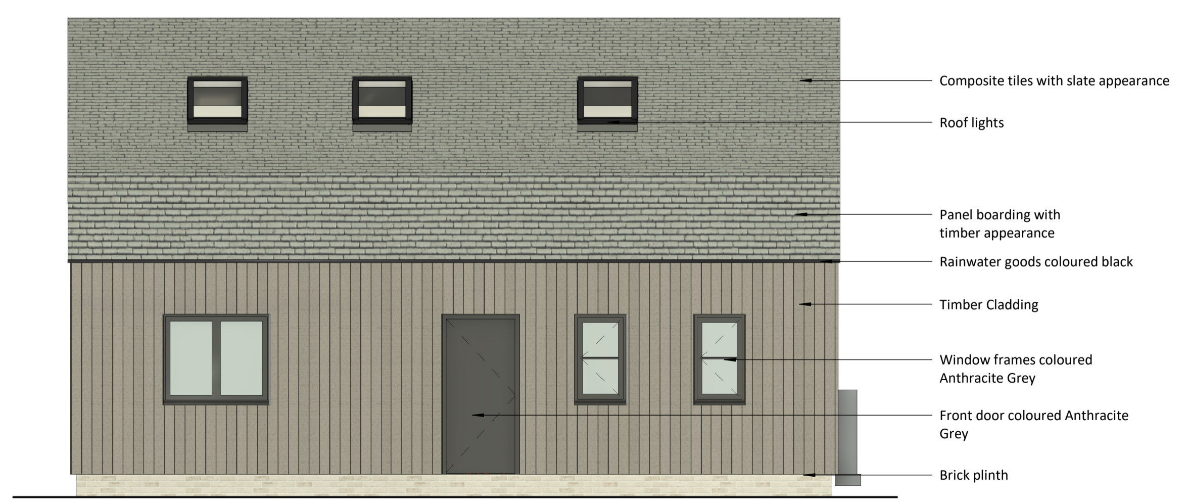
Front Elevation (North) 1 : 50
