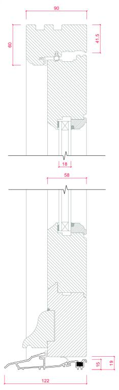
18mm Double Glazed Door - Open In Feature Mould: Ovolo Vertical Section Standard Aluminium Threshold
