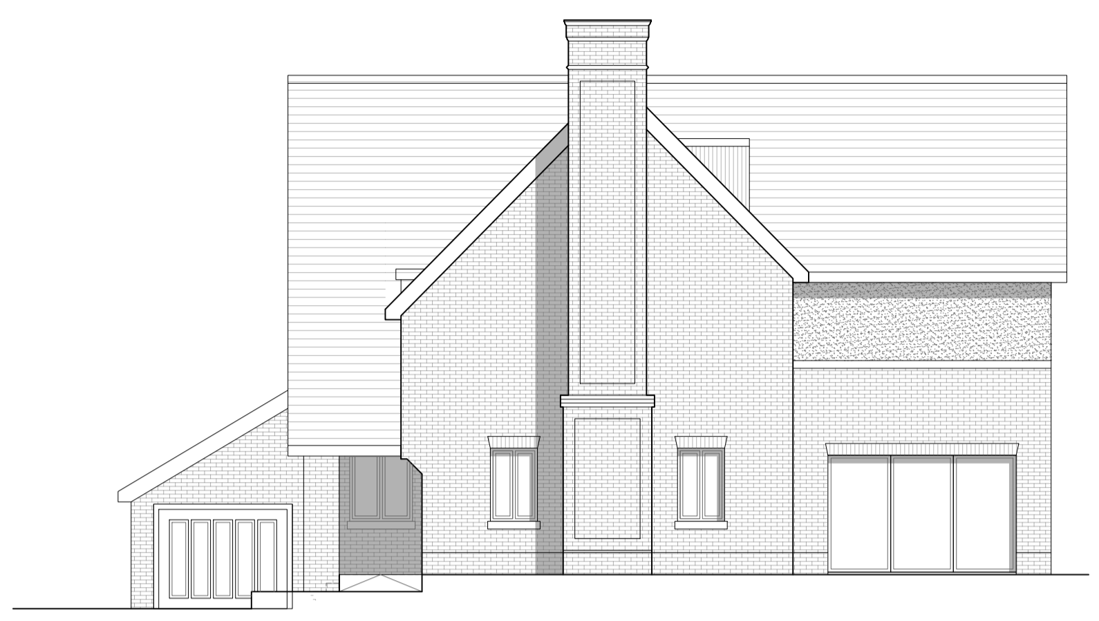
02 Proposed Side Elevation Scale 1:100 @ A1
