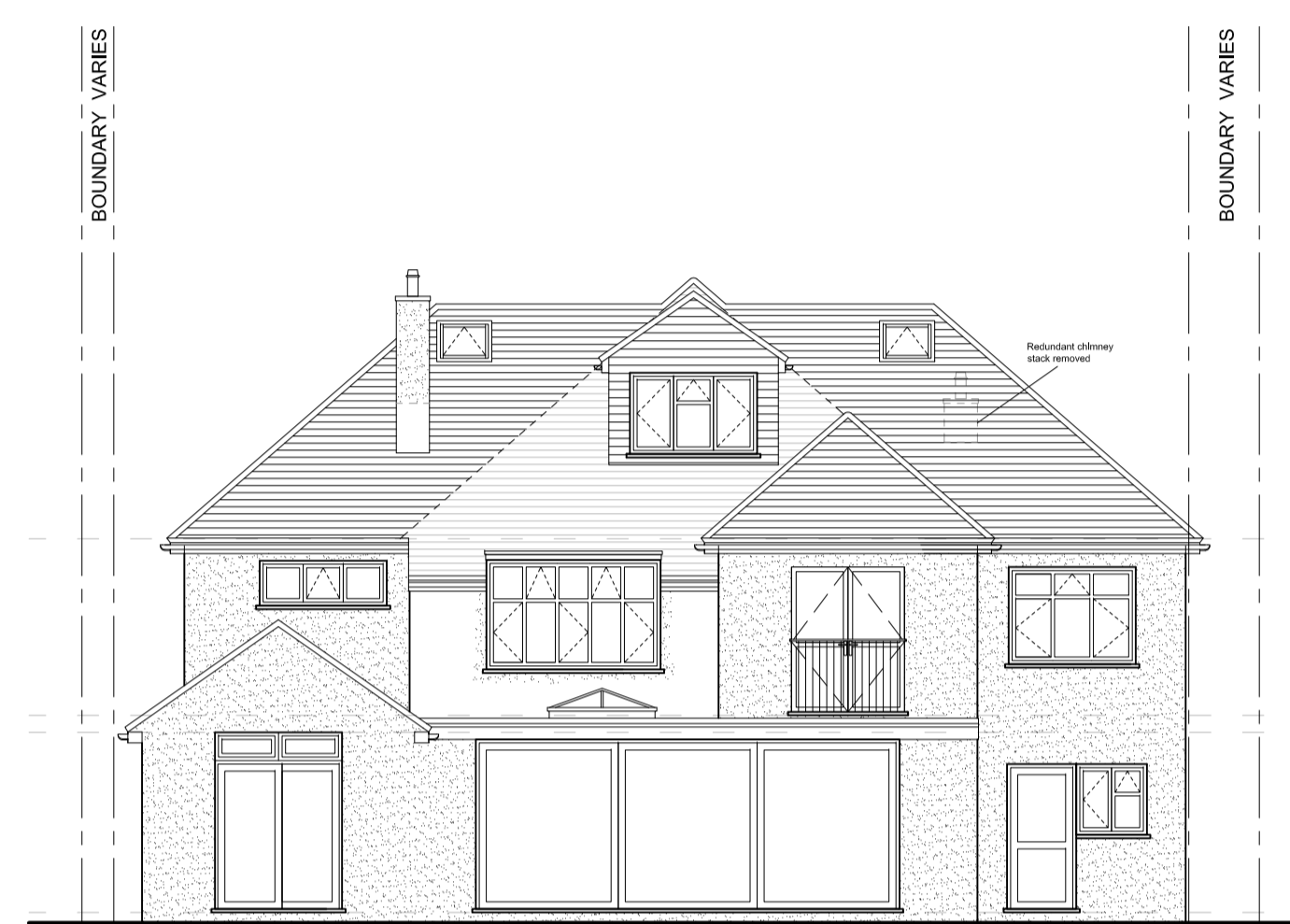
PROPOSED REAR ELEVATION
