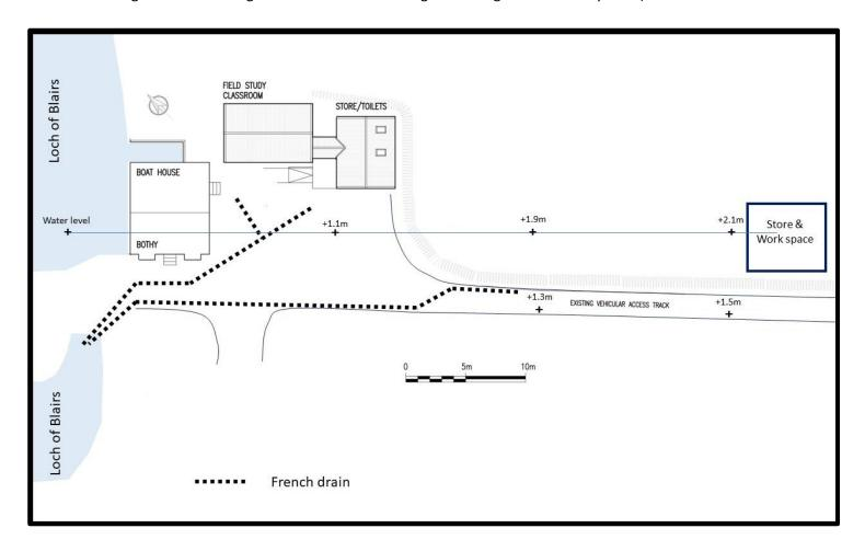
surface level) which terminates in the loch adjacent to the small secondary boat house. The French drain comprises of two 75mm diameter perforated pipes.
