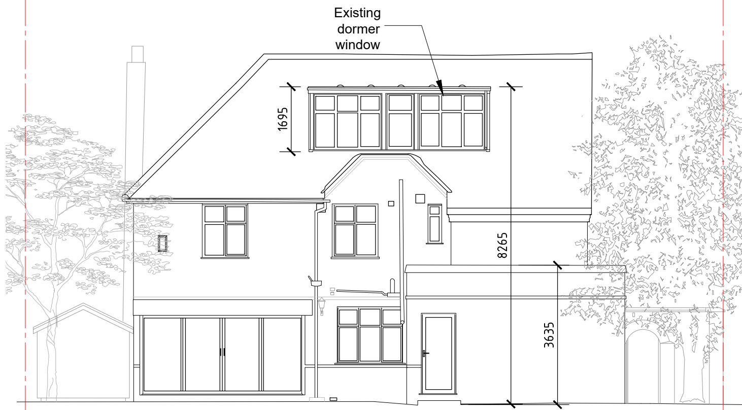
EXISTING REAR (WEST) ELEVATION Scale 1:100 @ A3
