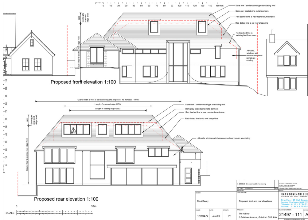
refused 23/P/01024 front and rear elevations – above
