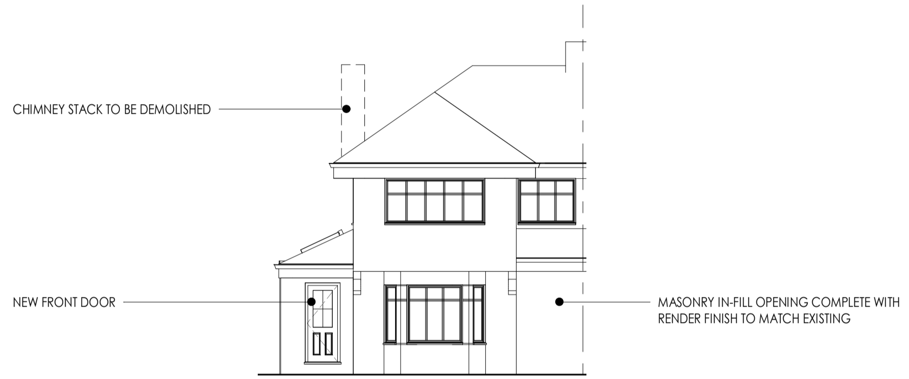
Front Elevation - Proposed 1 : 100
