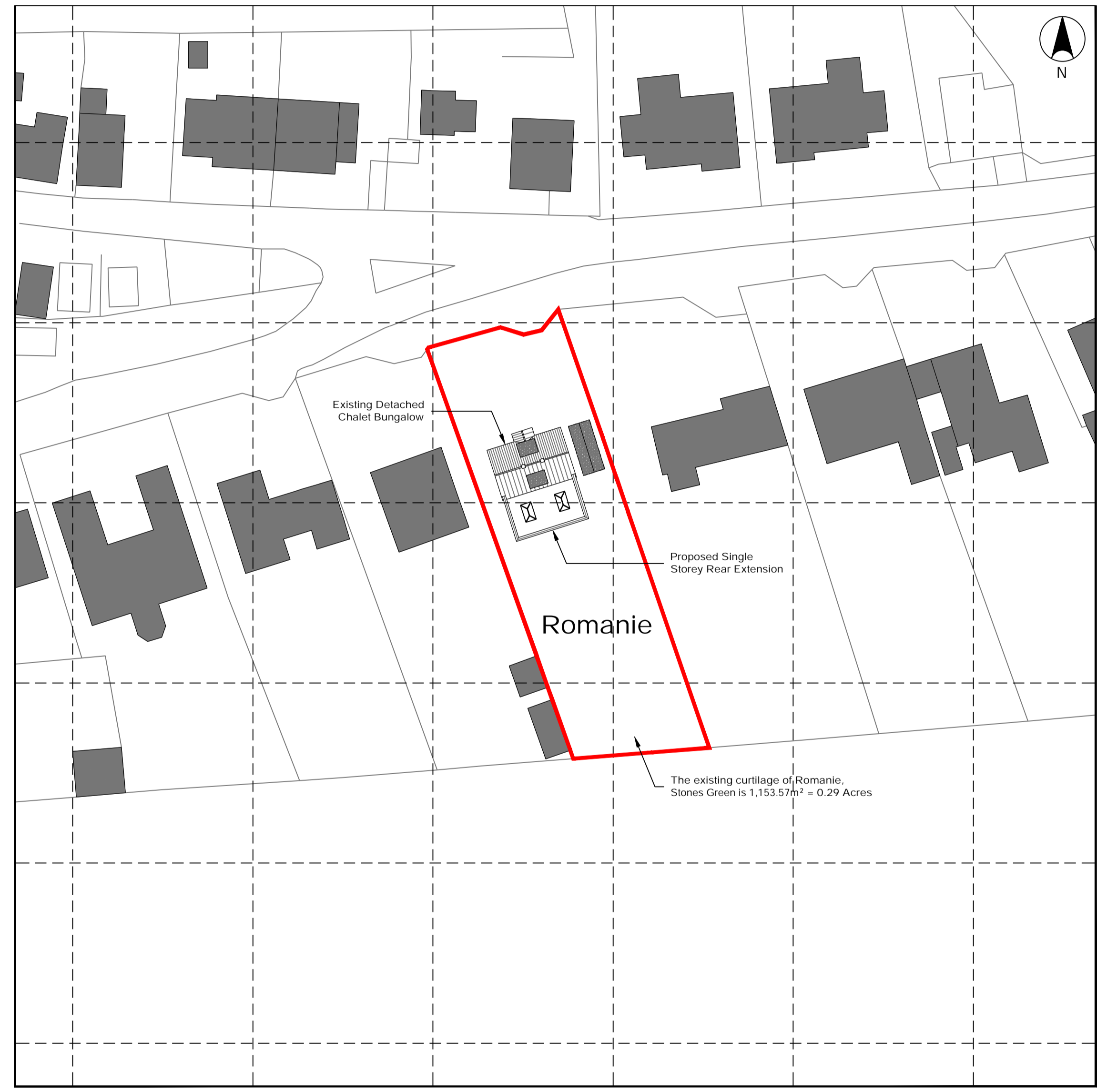
5.2 Proposed Block Plan Scale 1:500 0m 5m 10m 20m 30m 40m 50m 5m 15m 25m 35m 45m Scale 1:500 at A1 Site Location Key Red line: Indicates Boundary Line of Proposed Development Land Owned by the Applicant. Blue line: Indicates Boundary Line of Other Land Owned by the Applicant.
