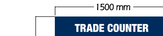
Sign 3b - 1no. fabricated aluminium sign with 30mm returns finished PMS 654 Blue with applied vinyl graphics. Cap Height = 110mm HTU = 3200mm
