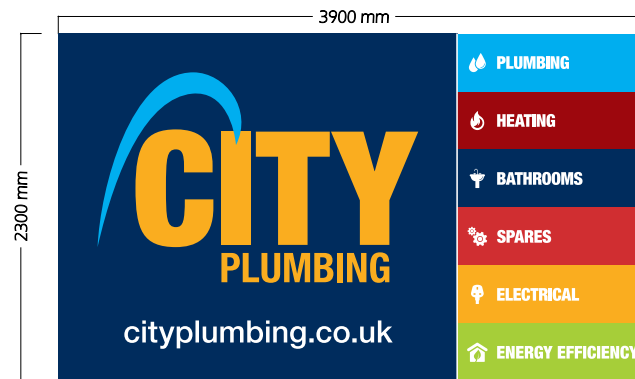
Sign 2 - 1no. Internally illuminated flex face sign finished PMS 654 Blue with digitally printed flexible face. Cap Height = 780mm HTU = 4000mm
