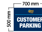
Sign 10 - 4no. flat 2mm aluminium sign with, finished PMS 654 Blue with applied vinyl graphics. Positions tbc.
