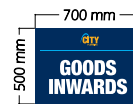
Sign 8 - 1no. flat 2mm aluminium sign with, finished PMS 654 Blue with applied vinyl graphics. Cap Height = 100mm HTU = 4800mm
