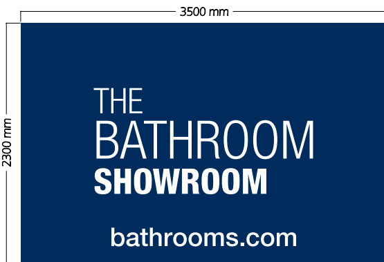
Sign 1 - 1no. Internally illuminated flex face sign finished PMS 654 Blue with digitally printed flexible face. Cap Height = 375mm HTU = 4000mm
