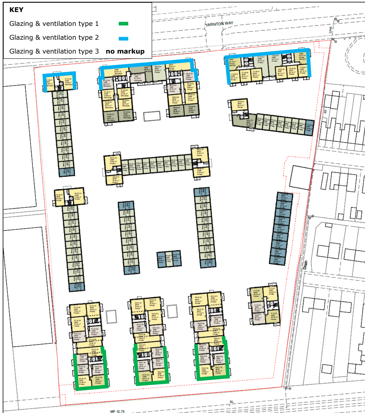
Figure 8-1: Glazing and Ventilation Layout (Residential)
