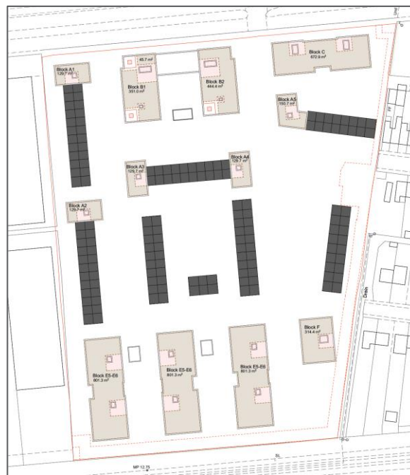
Figure 6: Roof area available for PV installation (Stockwool, 2023)
