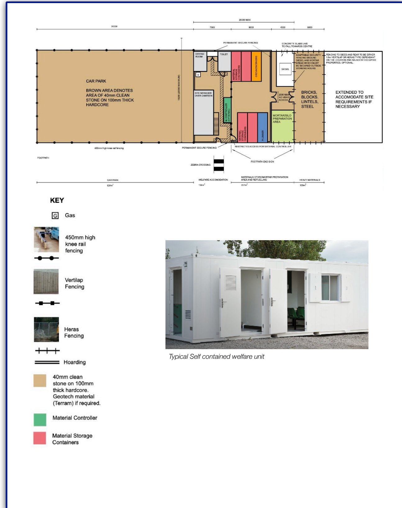
Fig. 4.2: Typical BHL Large Project Site Welfare, Parking & Storage Compound
