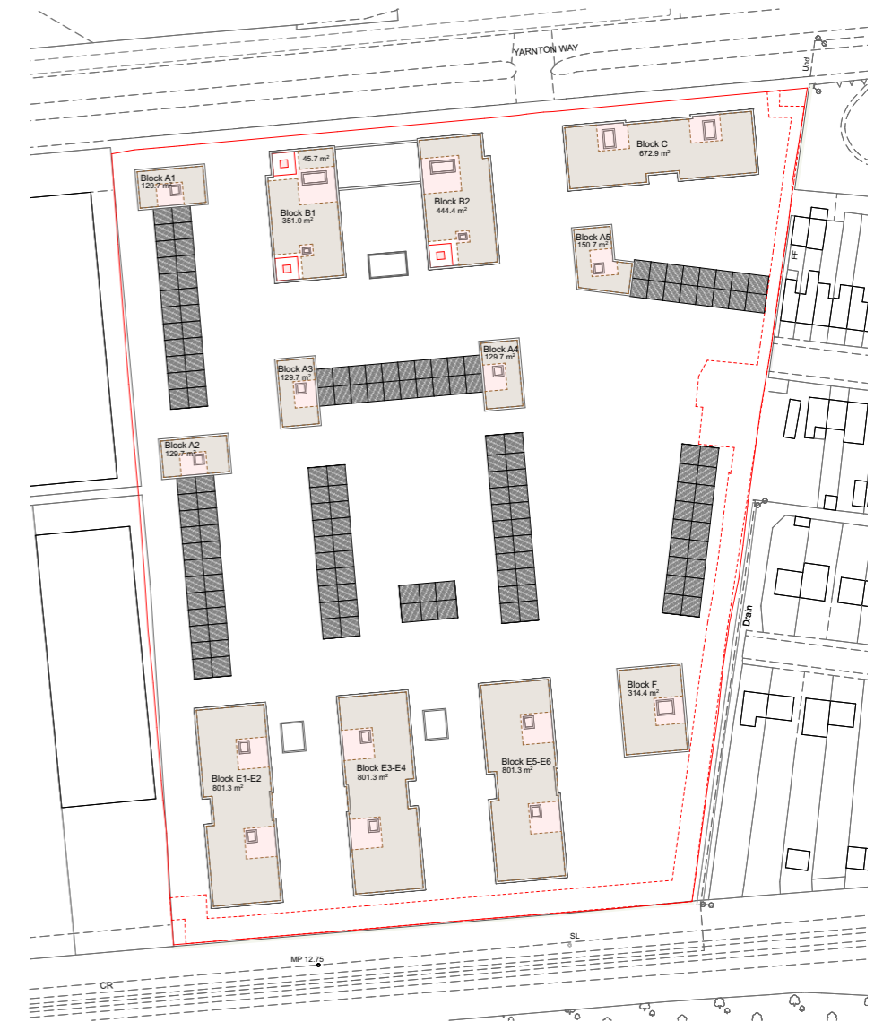
1. ROOF PLAN INDICATING AN AREA OF CIRCA 4,900m2 AVAILABLE FOR PV ARRAY
