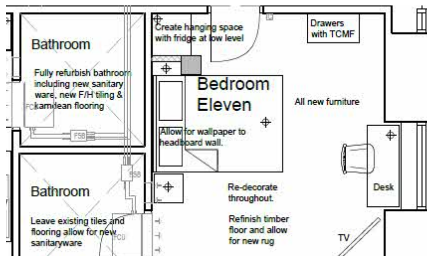
Above - First floor plan extract showing proposed location of fan coil and pipe runs for bedroom No 11
