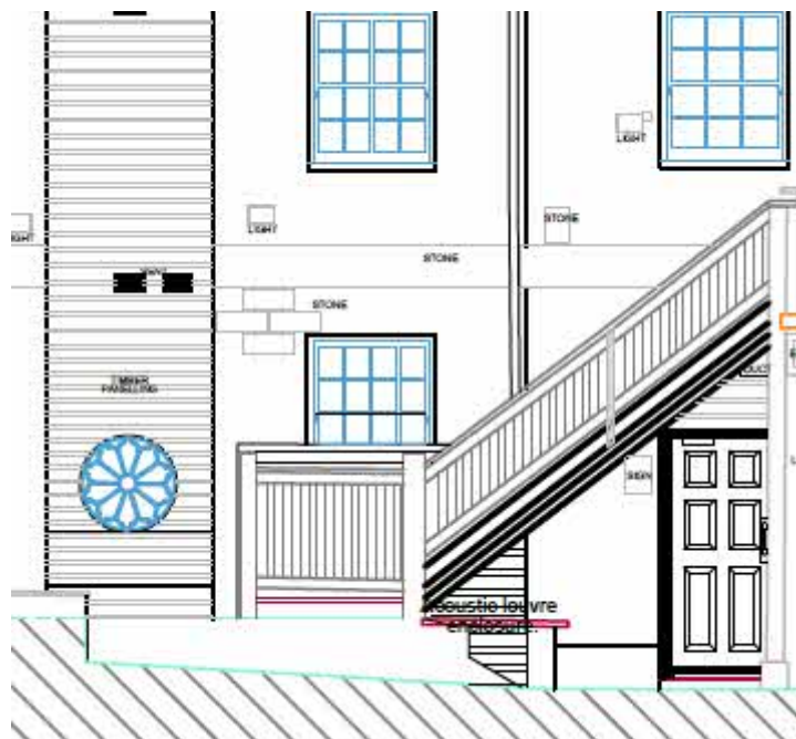
Above – Extract from proposed elevation plan showing position and scale of proposed louvred enclosure housing
