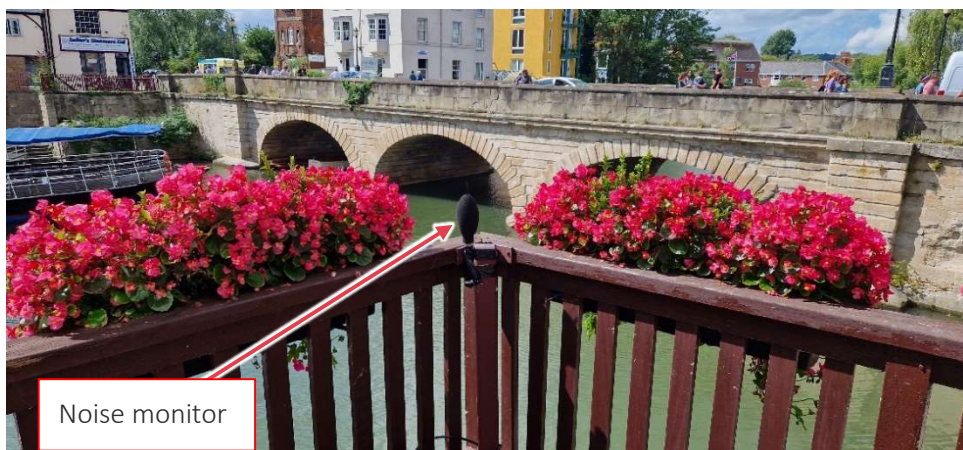
Figure 3-2: Photo taken on-site of noise monitor in place
