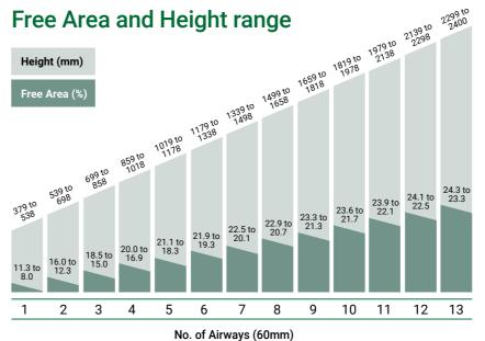
Free area shown is based on an 1150mm wide single piece louvre fitted with bird mesh and will vary slightly for different widths and bigger heights. Pressure losses for Class A rated louvres are available upon request.
