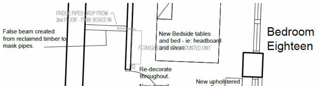
Above – Extract from proposed first floor plan of Wharf House and showing fan coil and pipe run positions of bedroom 18
