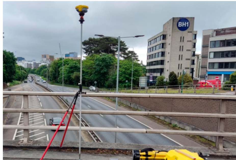
7: Field survey being carried out, GNSS receiver
