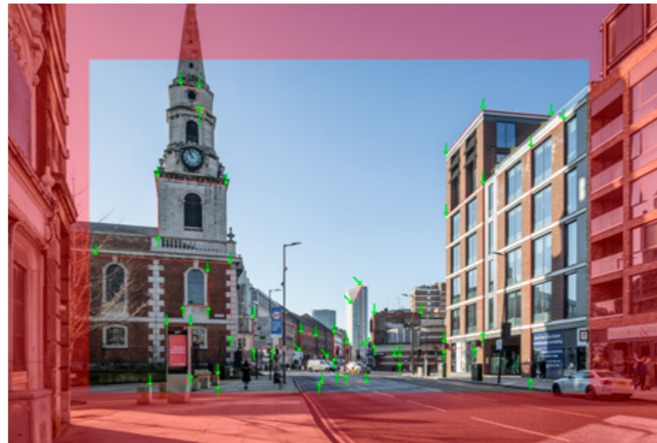
6: Background plate highlighting critical survey points in green and secondary survey strings in red
