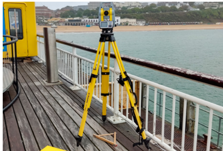
8: Field survey being carried out, total station
