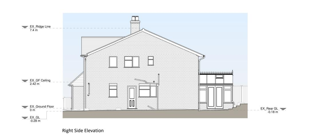
Existing Materials: Brickwork / Walls - Red brick and hung tiles Pitched roof - Slate/clay tiles Windows - White timber windows Doors - Green painted timber entrnace door and white uPVC conservatory RWP's / Gutter's / Fascia's - White uPVC
