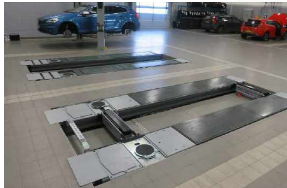
Example use of recessed vehicle lift in a column free space to maximise workshop flexibility
