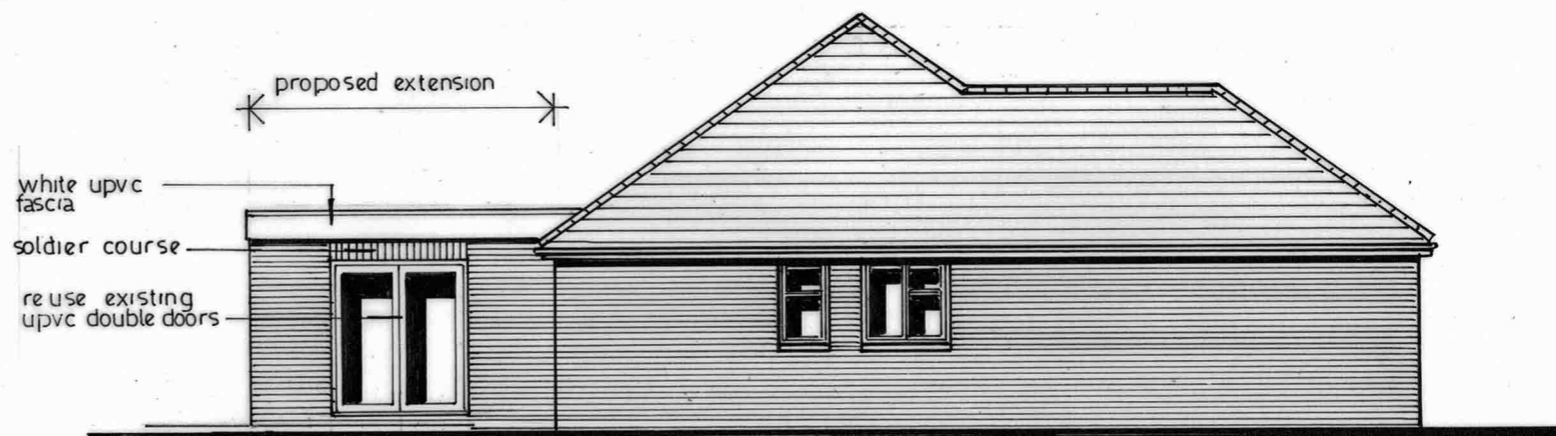
SIDE ELEVATION north west 1:100
