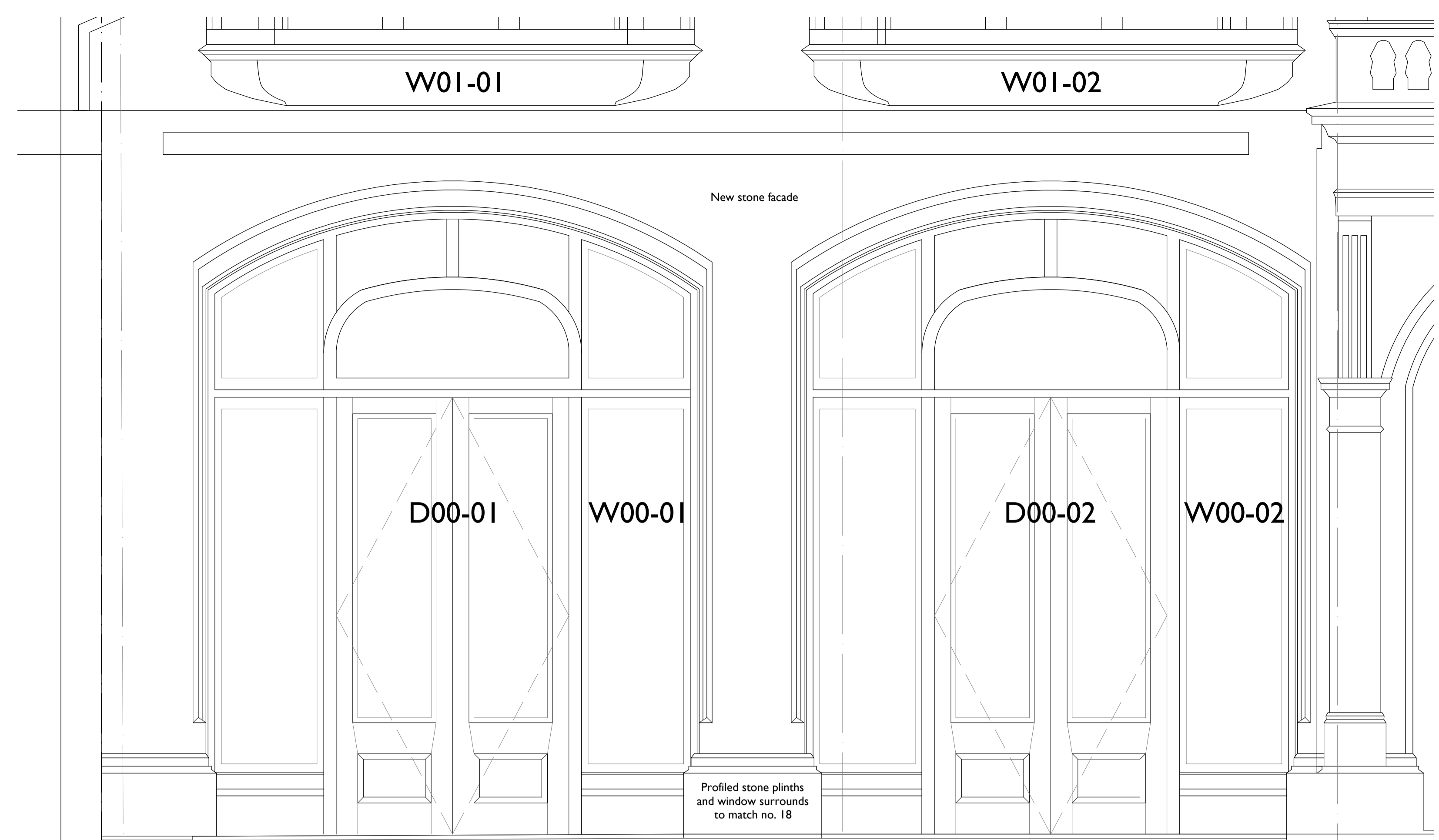
2 PROPOSED NEW SHOPFRONT ELEVATION 3028 1:20 @ A1
