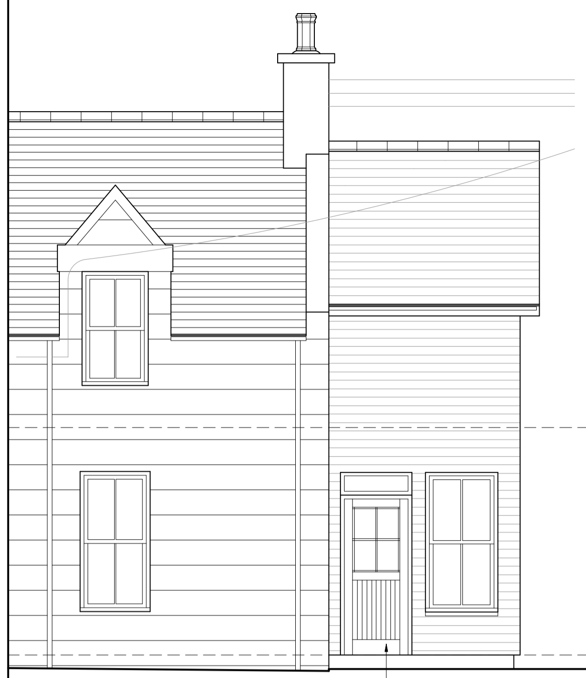
North-East Half glazed timber lined door with stain glass fanlight over
