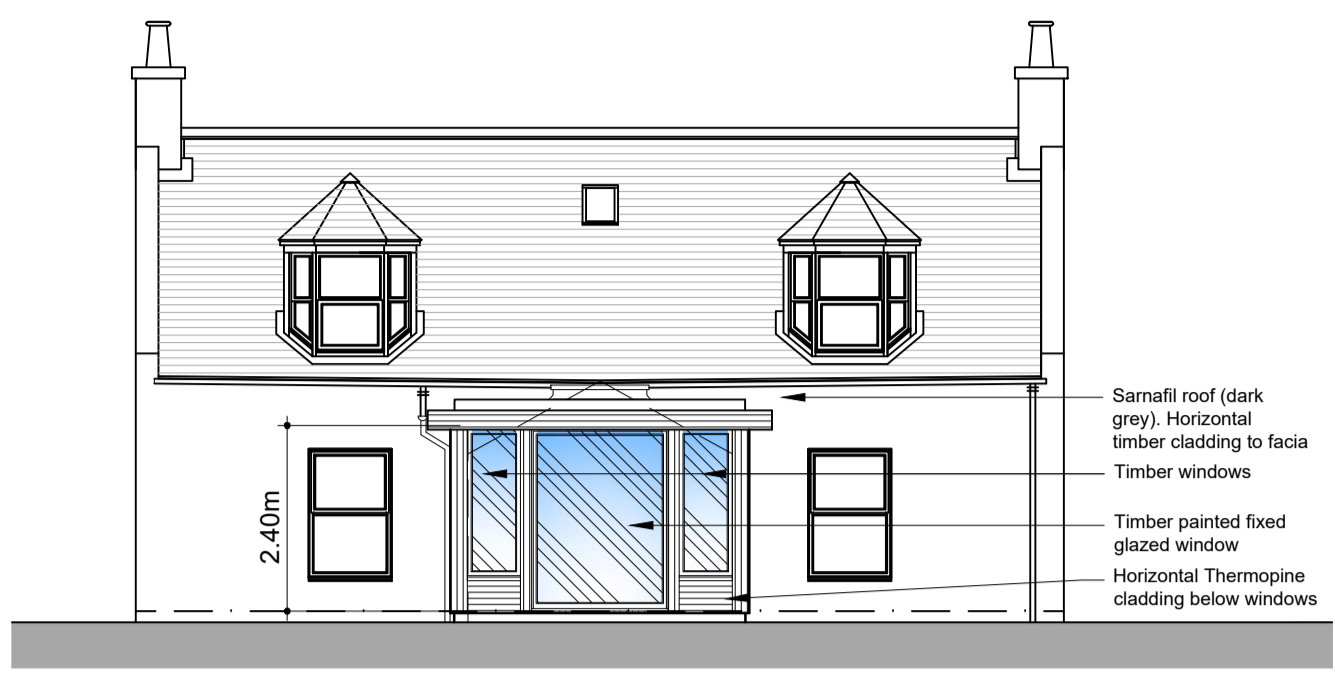
PROPOSED SOUTH EAST ELEVATION - SCALE 1:100
