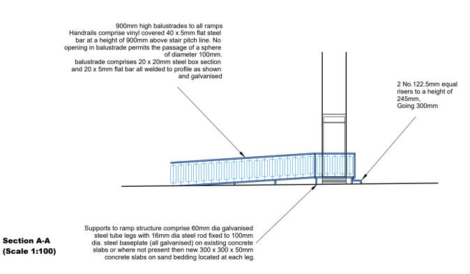
900mm high balustrades to all ramps Handrails comprise vinyl covered 40 x 5mm flat steel bar at a height of 900mm above stair pitch line. No opening in balustrade permits the passage of a sphere of diameter 100mm balustrade comprises 20 x 20mm steel box section and 20 x 5mm flat bar all welded to profile as shown
