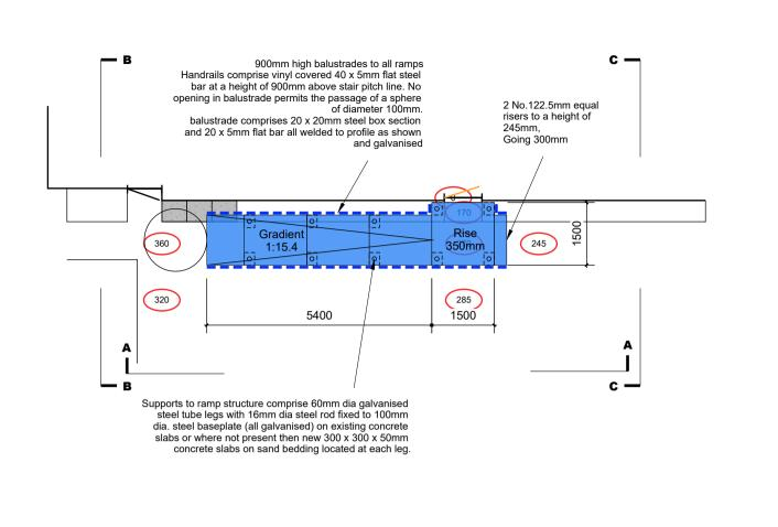
900mm high balustrades to all ramps Handrails comprise vinyl covered 40 x 5mm flat steel bar at a height of 900mm above stair pitch line. No opening in balustrade permits the passage of a sphere of diameter 100mm.
