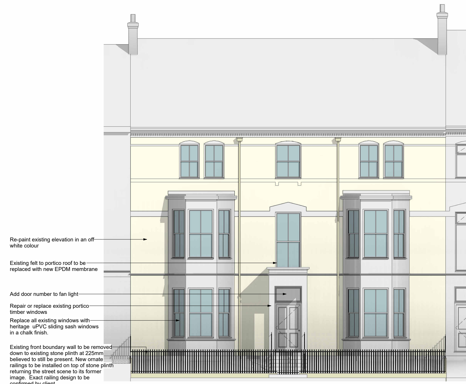
Proposed Front Elevation 1 : 100
