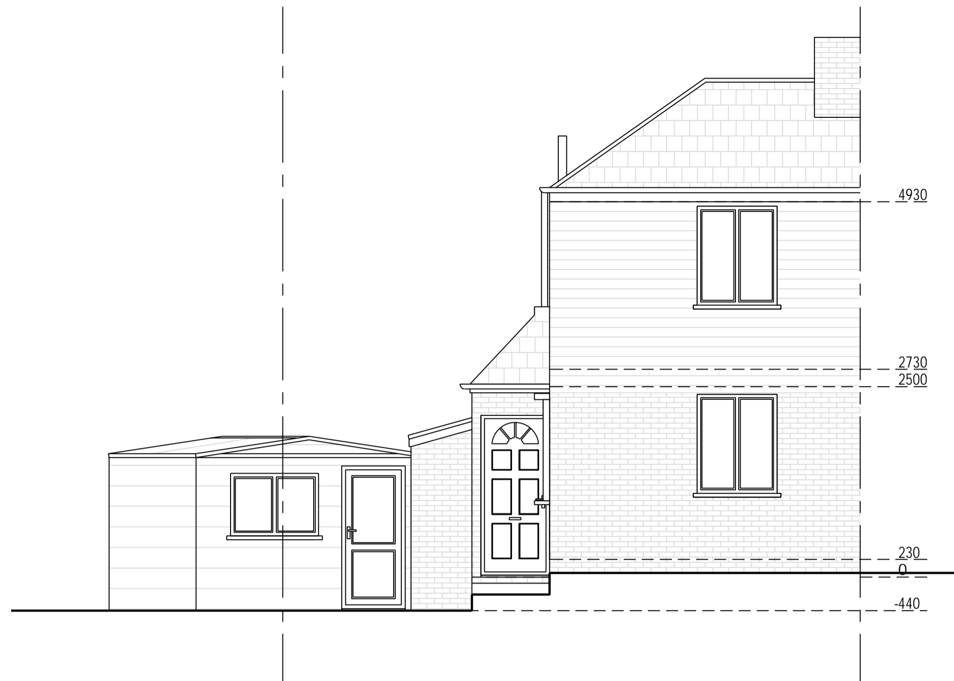
Existing Northwest Elevation Scale 1:50
