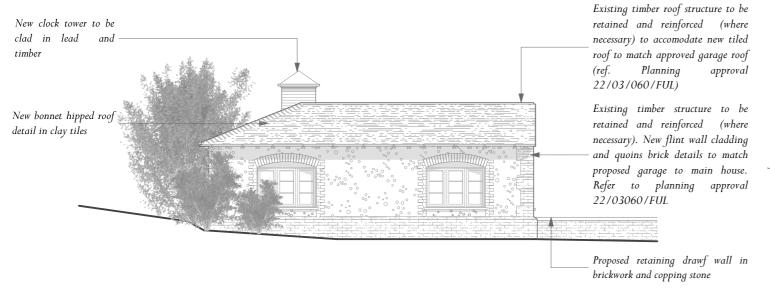
New clock tower to be clad in lead and timber boarding New low profile openable skylight fitted with anti-glare glass to reduce light spill Existing timber structure to be retained and reinforced (where necessary). New flint wall cladding and quoins brick details to match proposed garage to main house. Refer to planning approval 22/03060/FUL
