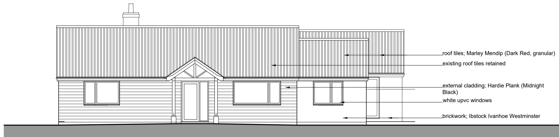
front elevation (north east)
