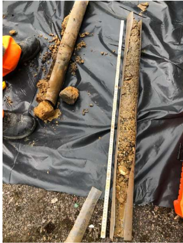
Photo 9 – Showing core samples taken from 1-3m bgl
