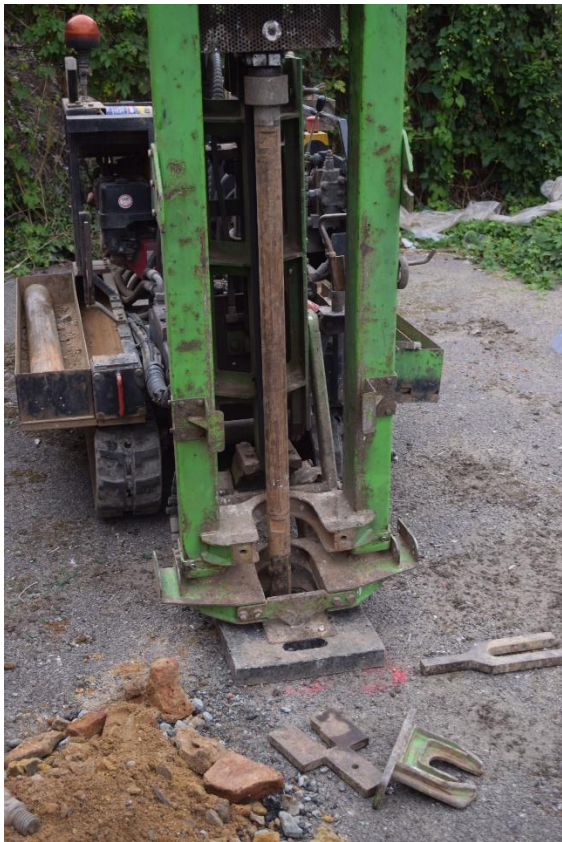
Plate 1. Working shot of Continuous Dynamic Sampler (CDS) rig cutting borehole WS01 (top) and WS03 and WS05 (bottom left and right respectively)
