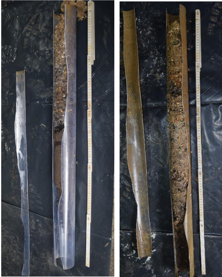
Plate 6. Split cores from borehole WS05: 1-2m (left) and 2-3m (right)
