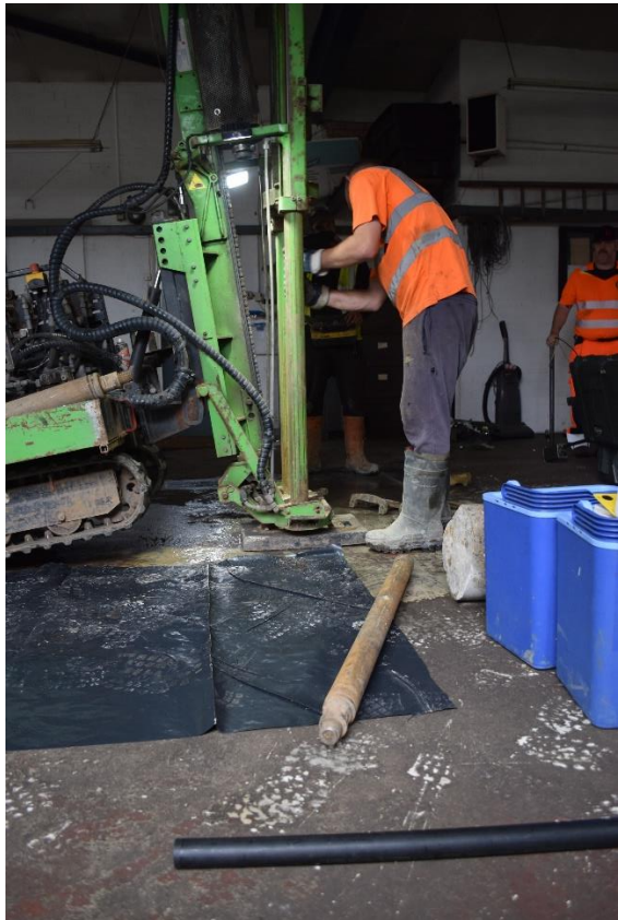
Plate 1. Working shot of Continuous Dynamic Sampler (CDS) rig cutting borehole WS01 (top) and WS03 and WS05 (bottom left and right respectively)
