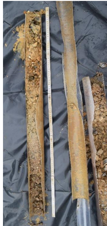
Plate 3. Split cores from borehole WS02: 1-2m (left) and 2-3m (right)
