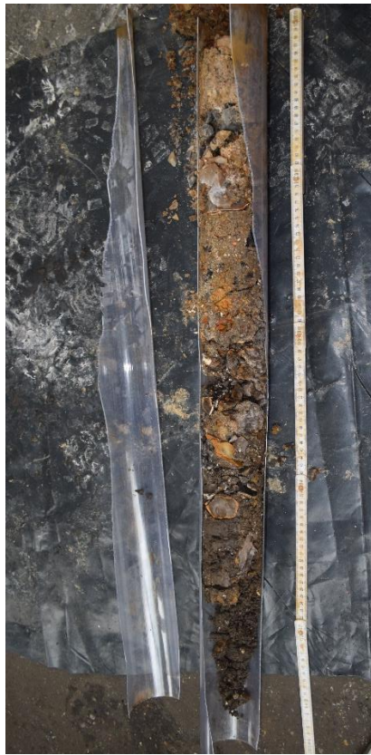
Plate 2. Split cores from borehole WS01: 1-2m (left) and 2-3m (right)
