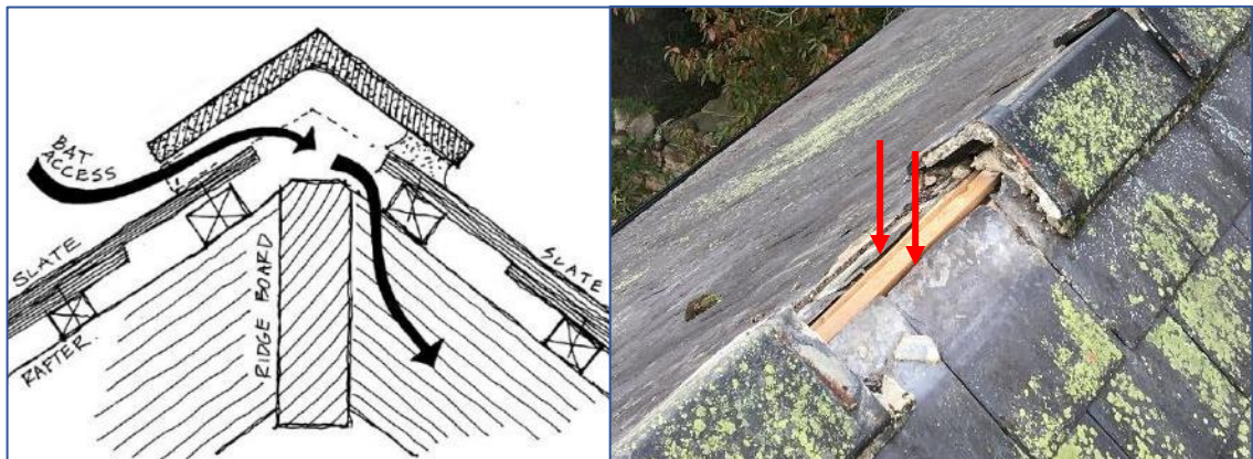
Figure D: Ridge board access.
