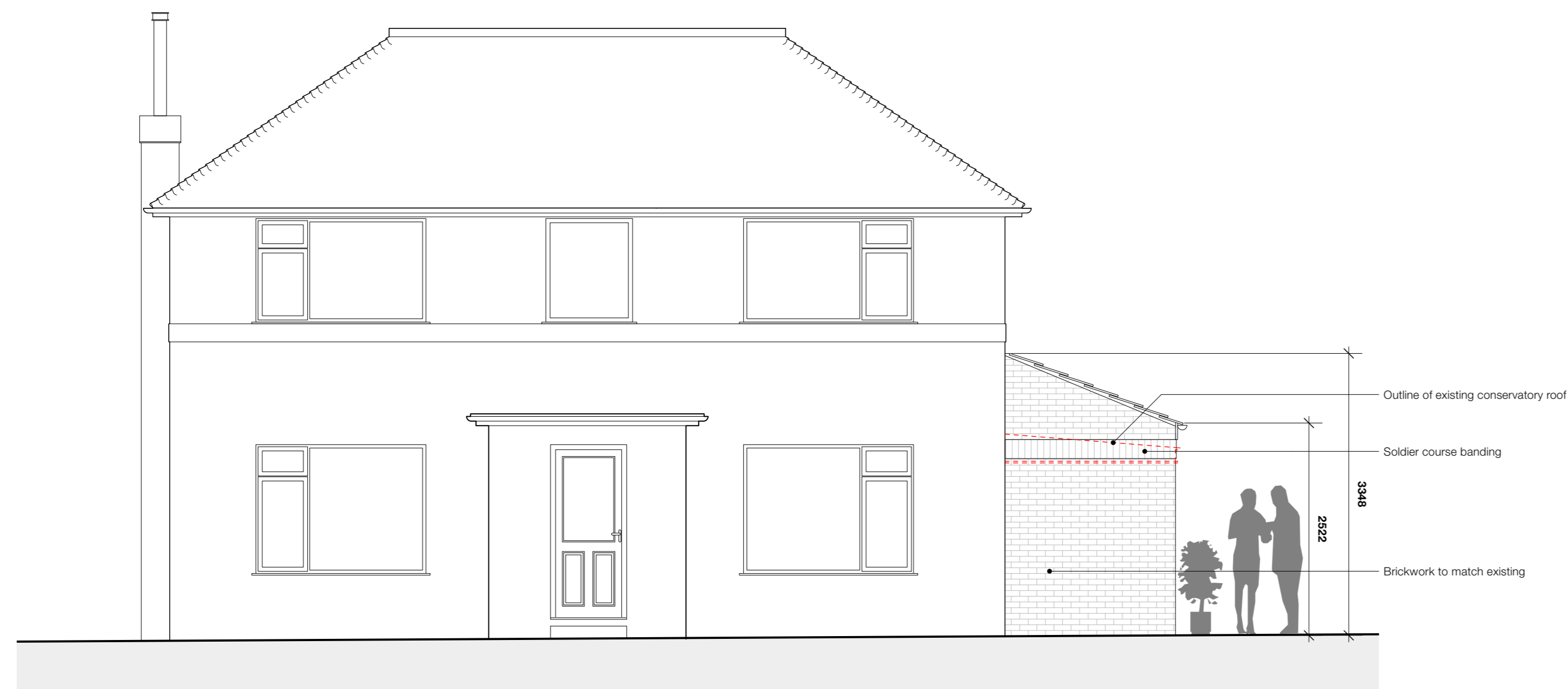
03 Proposed Front Elevation PL_02 Scale: 1:50
