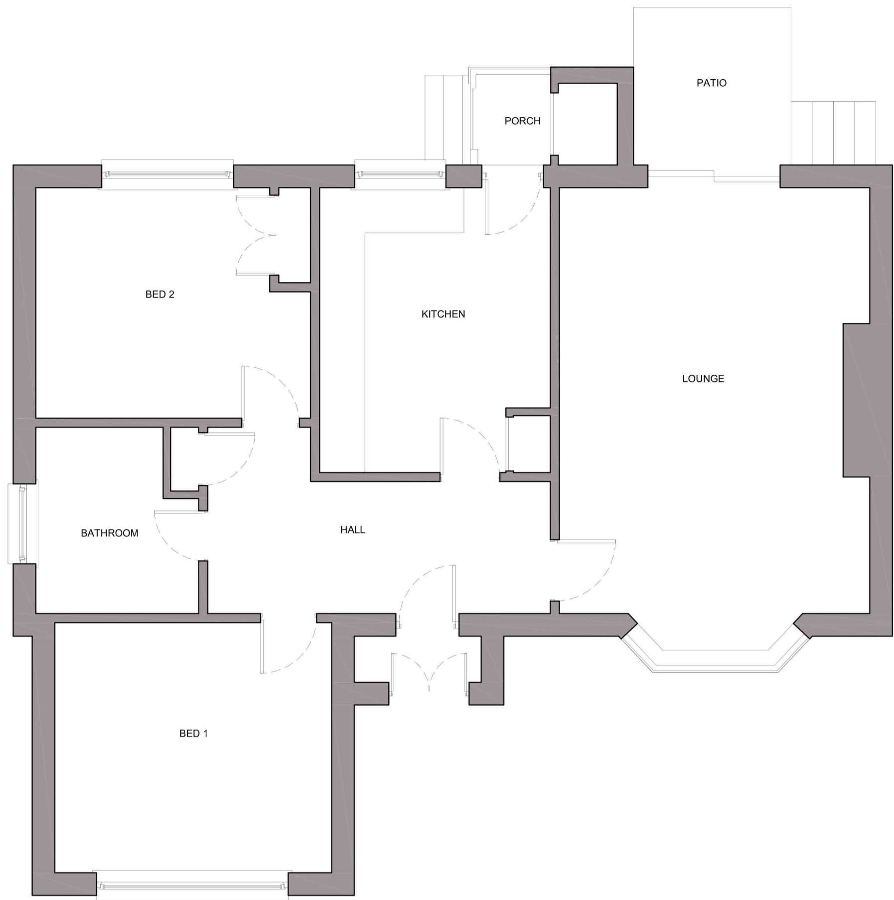
1:50 GROUND FLOOR WALL LAYOUT AS EXISTING
