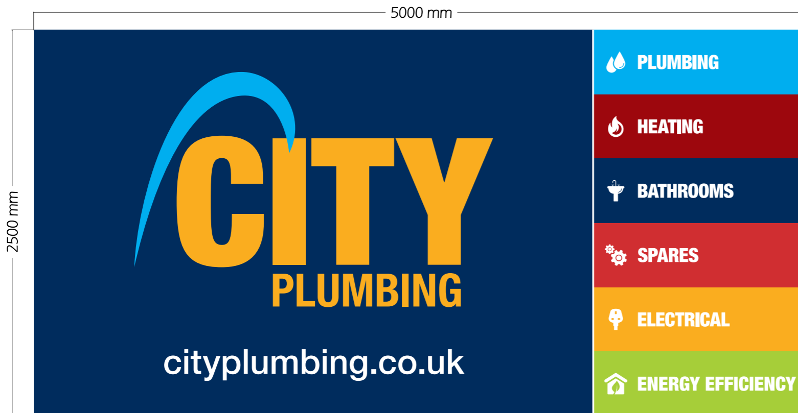
Sign 2 - 1 no. Internally illuminated flex face sign finished PMS 654 Blue with digitally printed flexible face. Cap Height = 850mm HTU = 5000mm
