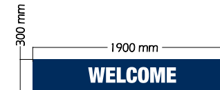
Sign 3 - 1no. fabricated aluminium sign with 30mm returns finished PMS 654 Blue with applied vinyl graphics. Cap Height = 150mm HTU = 2200mm
