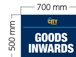
Sign 6 - 1 no. flat 2mm aluminium sign with, finished PMS 654 Blue with applied vinyl graphics. Cap Height = 100mm HTU = 4400mm
