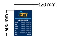
Sign 5 - 1no. fabricated aluminium sign with 30mm returns finished PMS 654 Blue (OPENING TIMES TBC) Cap Height = 75mm HTU = 1000mm
