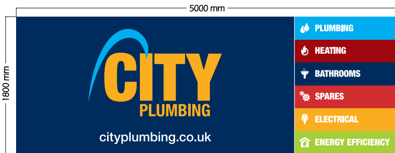
Sign 1 - 1no. Internally illuminated flex face sign finished PMS 654 Blue with digitally printed flexible face. Cap Height = 620mm HTU = 5000mm
